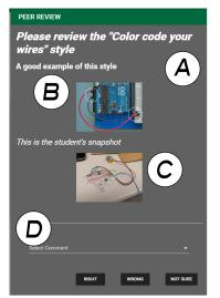
Figure 6: The Peer Review Interface; (A) Name of particular circuit style to be evaluated; (B) Photograph example of good style implementation; (C) Photograph submitted by fellow student to be reviewed; (D) Student feedback options.
