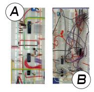
Figure 2: (A) Example of good circuit style: wires go around ICs instead of over, components lay flat against board, etc. (B) Example of poor circuit style: wires long and tangled, components crammed together, etc.
