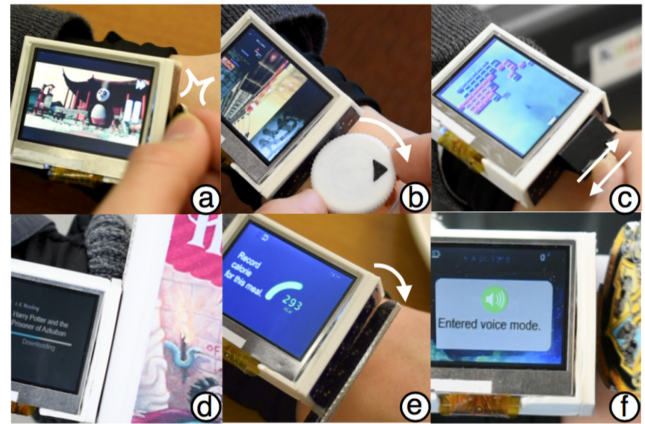
Figure 15. Inductivo demo applications: (a) video player, (b) aircraft game, (c) brick breaker game, (d) audio book app, (e) fitness app, (f) setting voice mode app.
