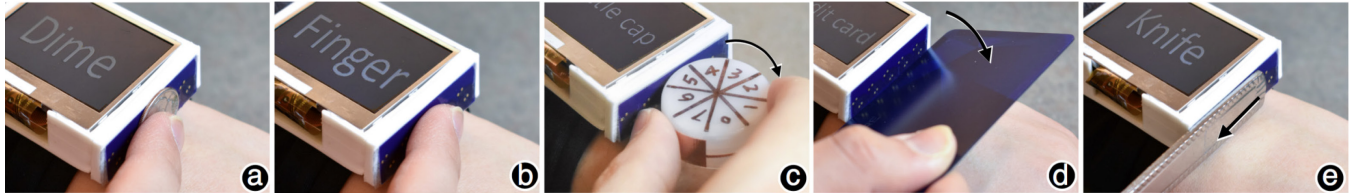
Figure 1. Indutivo recognizes the tap of a conductive objects on a smartwatch, such as (a) a dime, or (b) finger. It can sense (c) the rotation of a bottle cap instrumented using copper tape, (d) hinge of a metal credit card, and (e) slide of the handle of a table knife.
